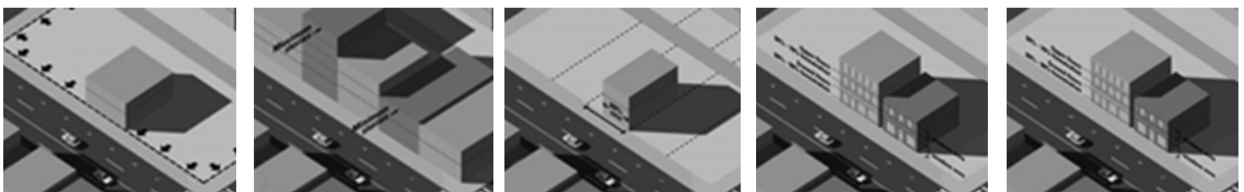
Figure 3. 1. building line; 2. maximum and minimum height; 3. minimum width of the elevation in relation to the width of the plot; 4. surface area of windows in relation to the surface of the elevation (on individual storeys); 5. other attributes, including greenery and street furniture
